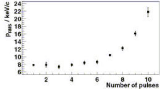
Figure 4: Momentum spread as function of the number of pulses in the laser bunch train at a bunch charge of about 0.4 nC.
