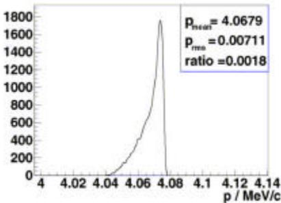
Figure 3: Momentum distribution for a gradient of about 35 MV/m and a mean charge of about 0.4 nC.
