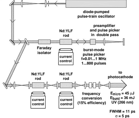
Figure 2: Optical scheme of the current PITZ laser.
