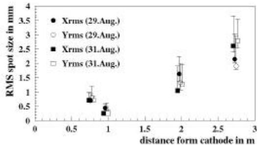
Figure 5: Two measurements of beam spot sizes along the beam line under similar operation conditions. The measurements at each of the four locations are slightly displaced to show them more clearly.
