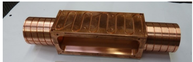
Figure 3: Copper heat conducting elements.
