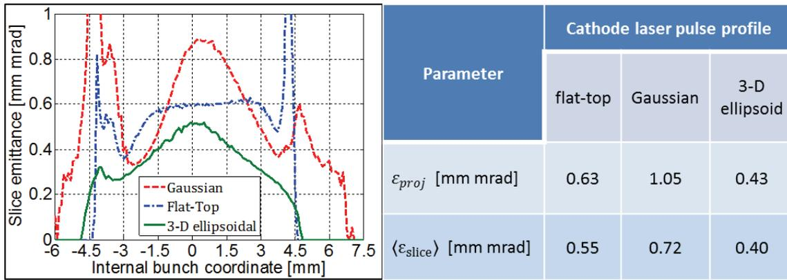
Figure 1: Beam dynamics simulation of electron bunches for photo cathode laser pulses with flat-top, Gaussian and 3-D ellipsoidal temporal profiles; left: normalized transverse slice emittance  $\epsilon_{slice}$  distribution along the electron bunch; right: values of normalized transverse projected emittance  $\epsilon_{proj}$  and normalized average slice emittance  $\langle \epsilon_{slice} \rangle$ .
