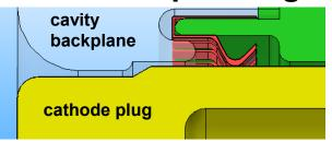
+ spring insert can be exchanged
