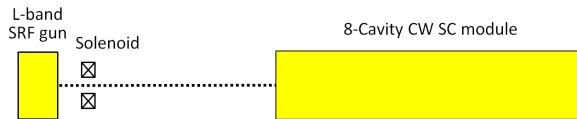
Figure 4: L-band superconducting RF gun based CW photoinjector layout (preliminary example, not optimal).
