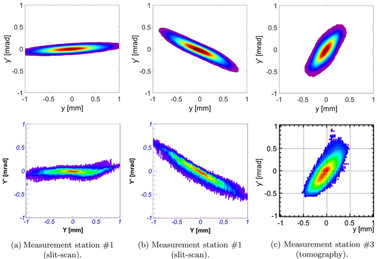
**Fig. 4.** Simulated (top) and measured (bottom) vertical trace-space distributions at the three measurement stations. The colour code represents normalized charge density (maximum is red, minimum is violet). (For interpretation of the references to colour in this figure caption, the reader is referred to the web version of this paper.)
