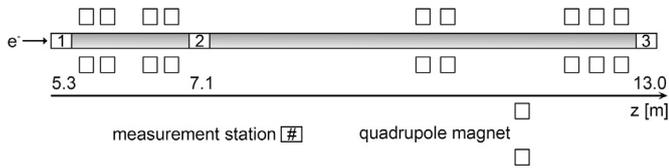
**Fig. 1.** Schematic layout of the matching lattice used for the PST measurement at PITZ. Nine matching quadrupoles are located among three transverse emittance measurement stations, the longitudinal position of which is indicated on the coordinate axis below.
