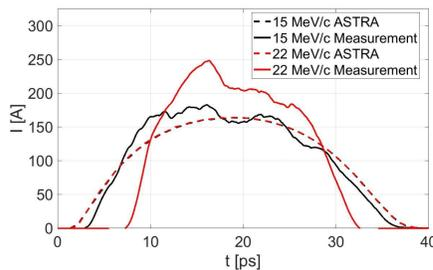
Beam current profiles of the optimized 4 nC beams. Note that the profiles from ASTRA are for the beams at  $Z = 5.28 \text{ m}$ .
