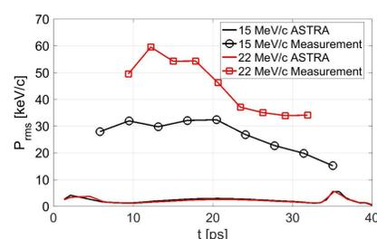
Slice momentum spread profiles of the 4 nC beams. Note that the profiles from ASTRA are for the beams at  $Z = 5.28 \text{ m}$ .
