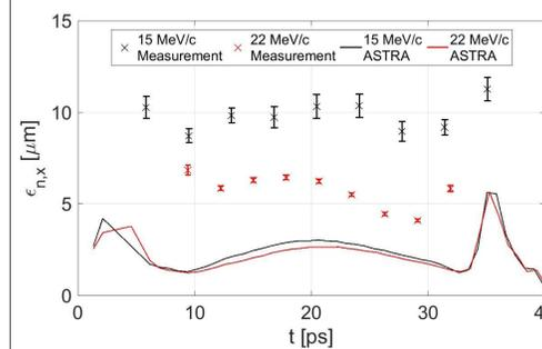
Horizontal slice emittance of the optimized beams at  $Z = 5.28 \text{ m}$ . The error bars only include statistical errors.
