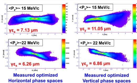
The transverse projected emittance is measured using the single slit-scan technique. Slit masks with an opening gap of 10  $\mu\text{m}$  and a beamlet collecting screen locate at  $Z = 5.28 \text{ m}$  and  $Z = 8.41 \text{ m}$ , respectively.
