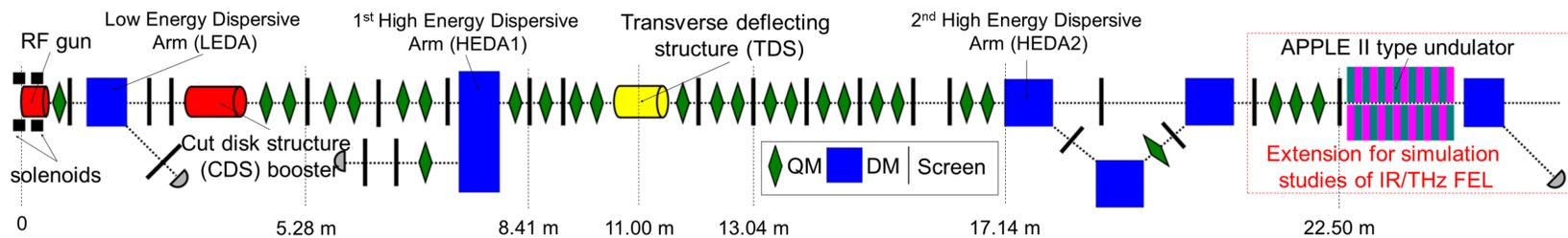
Layout of the PITZ beamline including extension for an IR/THz FEL for simulation studies. Here QM, DM and screen represent quadrupole magnets, dipole magnets and screen stations for monitoring of beam transverse profiles, respectively. The numbers represent the distance from the photocathode location ( $Z = 0$ ).
