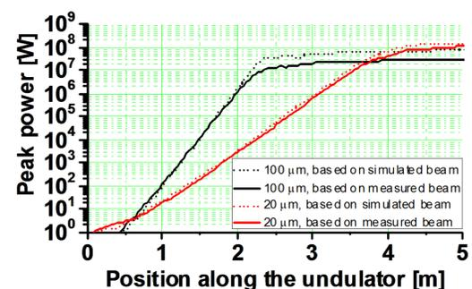
Simulated FEL peak powers along the undulator axis.
