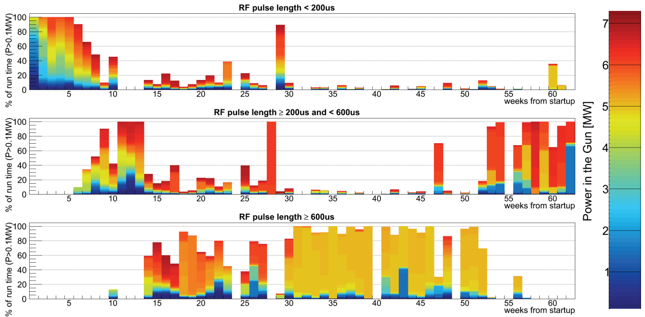
Figure 5: Weekly percentage of gun 4.2 operation time spent at different RF pulse lengths. The color code provides further information about the time spent at different power levels.
