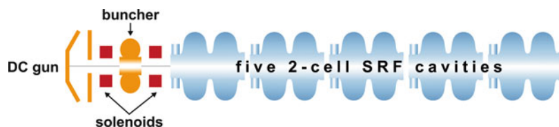
Fig. 6 Schematic of the photoelectron injector for the Cornell ERL-based X-ray source
