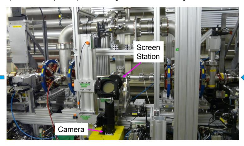
Best result: <100μm spot size (100 pC bunch charge; 22 MeV; no scattering foil)</p>
