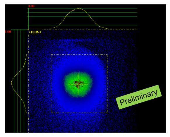
Capturing of tightly focused beam behind plasma cell (at that time only 2 Quads available for beam capturing)
