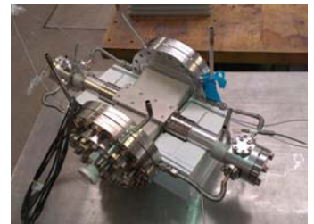
The completed plasma cell. The big side ports allow the coupling of the ionization laser which generates the plasma channel at the center of the Lithium column and leave additional space for plasma diagnostics.
