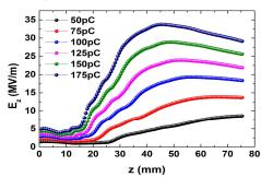
Above Fig. shows that the peak accelerating field occurs earlier for greater bunch charges, indicating a more rapid growth of the self-modulation instability. As the self-modulation instability grows,  $E_z$  saturates and the saturation distances decreases from 70mm to 40mm with increasing charge. The simulation result also indicates that within the propagation distance of z=15mm,  $E_z$  remains almost constant.
