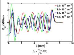
Where R(0) is a unitless transverse geometrical factor. R(0) is an increasing function of  $k_p\sigma_r$ , the bunch transverse size  $\sigma_r$  relative to the plasma skin depth  $c/\omega_p$ . At 5mm distance the amplitude of longitudinal wakefield  $E_x$  decreases from 2 to  $0.5\,MV/m$  as the plasma density  $n_p$  is increased, indicating the dominance of the decreasing term  $1/\sqrt{n_p}$  over the increasing term R(0).
