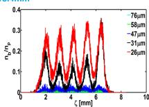
Smaller beam size expels plasma electron more strongly, generating strong transverse wakefields which in turn modulate beam energy strongly.
