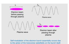
In its simplest form of self-modulation, a long charge particle beam  $(L>\lambda_p)$  when propagates through the plasma generates a wake within its body due to perturbation of plasma, which modulates the beam itself, leading to the positive feedback and unstable modulation of the whole beam along the propagation direction. This self-modulation splits the long beam into short bunches of length  $\lambda_p$ , which resonantly drive the plasma wake. The longitudinal electric field is given by
