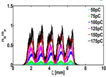
The density modulation is small for lower charge (50pC). On the contrary, for the high charge case where Q=175pC, the electron bunch starts modulating into small beamlets on the scale of the plasma wavelength, drives the plasma wakefield resonantly.
