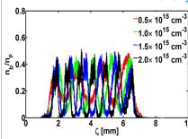
Above Fig. shows the snapshot of the beam density modulation at 15.4mm in the plasma with different plasma densities when charge and beam size are kept constant. With different plasma densities  $(n_p)$  the period of modulation changes since  $\lambda_p \propto 1/\sqrt{n_p}$ .
