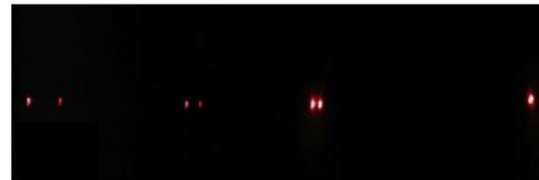
Diffraction pattern for the 670 nm and 632.8 nm. From right to left 0 th , 1 st , 2 nd ... order diffraction pattern. 0 th order diffraction overlaps for both lasers because it is just a reflection from grating.
