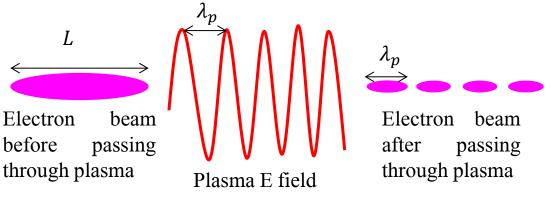
A long  $(L > \lambda_p)$ , relativistic particle beam propagating in an overdense plasma is subject to the self-modulation instability via transverse wakefields of plasma wave.
