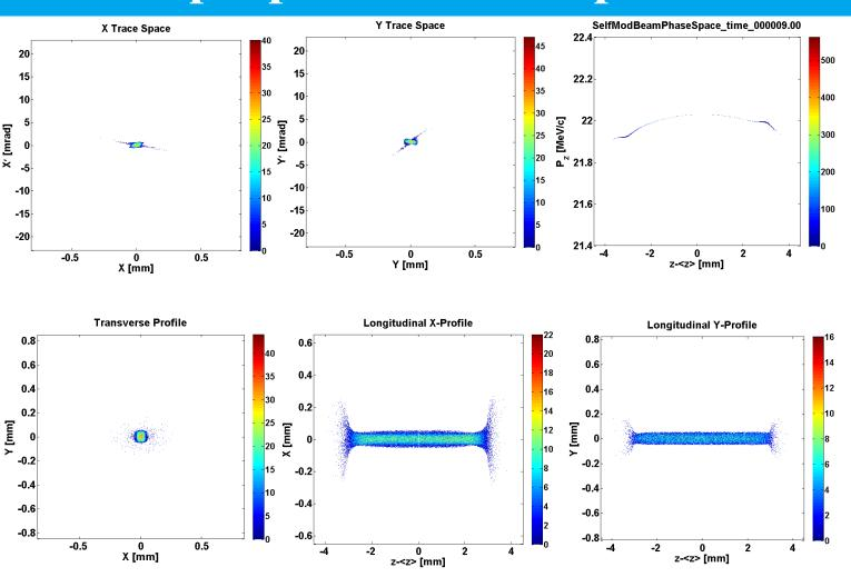
x'=1.6mrad y'=1.6mrad  $P_z^{mean}=22MeV/c$   $P_z^{rms}=22MeV/c$   $x_{rms}=27\mu m$   $y_{rms}=26\mu m$   $\varepsilon_x=0.370mm\ mrad$   $\varepsilon_y=0.375mm\ mrad$
