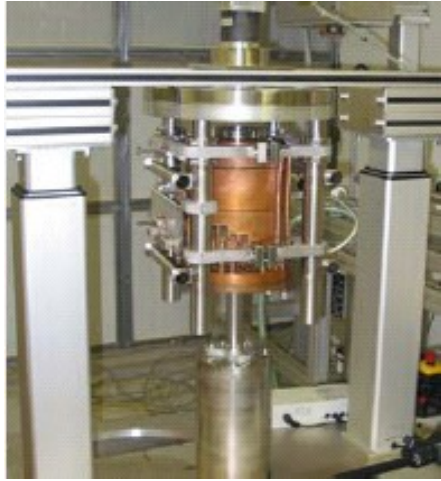
Vertical cleaning setup with 110° rotating nozzle.
