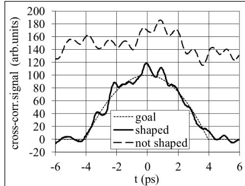
Figure 4: Scanning cross-correlator measurements of pulses w/o pulse shaping (dashed line), w/- amplitude mask pulse shaping (solid line) and aspired profile (dotted line).
