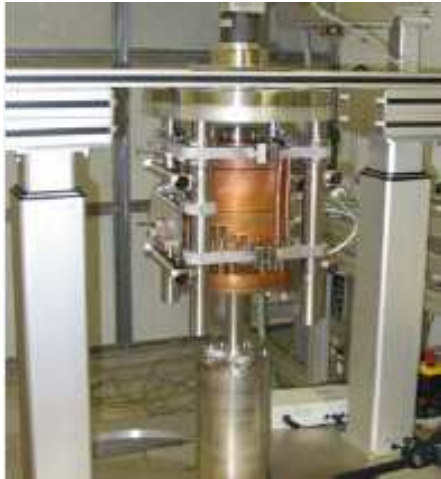
Vertical cleaning setup with 110° rotating nozzle.
