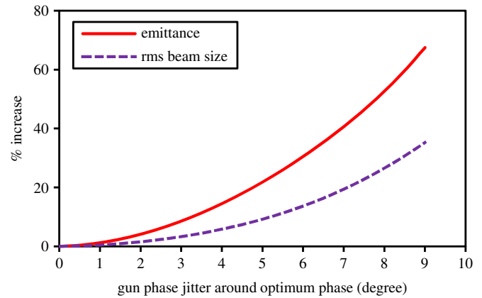
Fig. 26. Simulated emittance and beam size increase due to gun phase jittering (peak-to-peak) for a charge of 1 nC per bunch. Machine and beam parameters used in this simulation are the same as for the simulation in Fig. 15.
