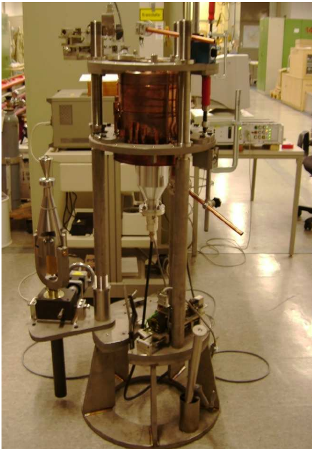
Figure 2: Photograph of the tuning device with the gun cavity, the BESSY test coupler, the bead pull setup, and the tuning tools: the clamp (mounted) and the stamp.
