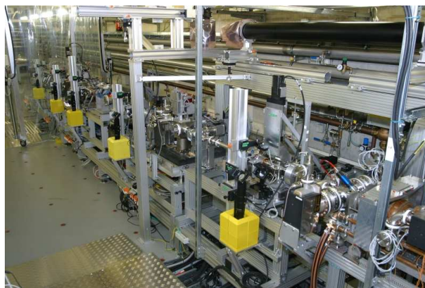
Figure 1: Photograph of the PITZ1.6 beamline after the booster with the new emittance measurement systems.
