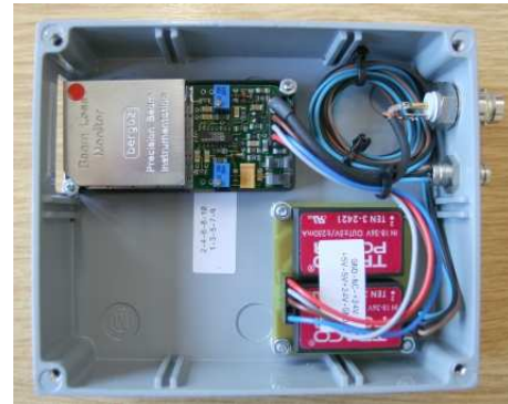
Figure 8: Photograph of the BERGOZ BLM mounted in iron housing together with needed electronics.
