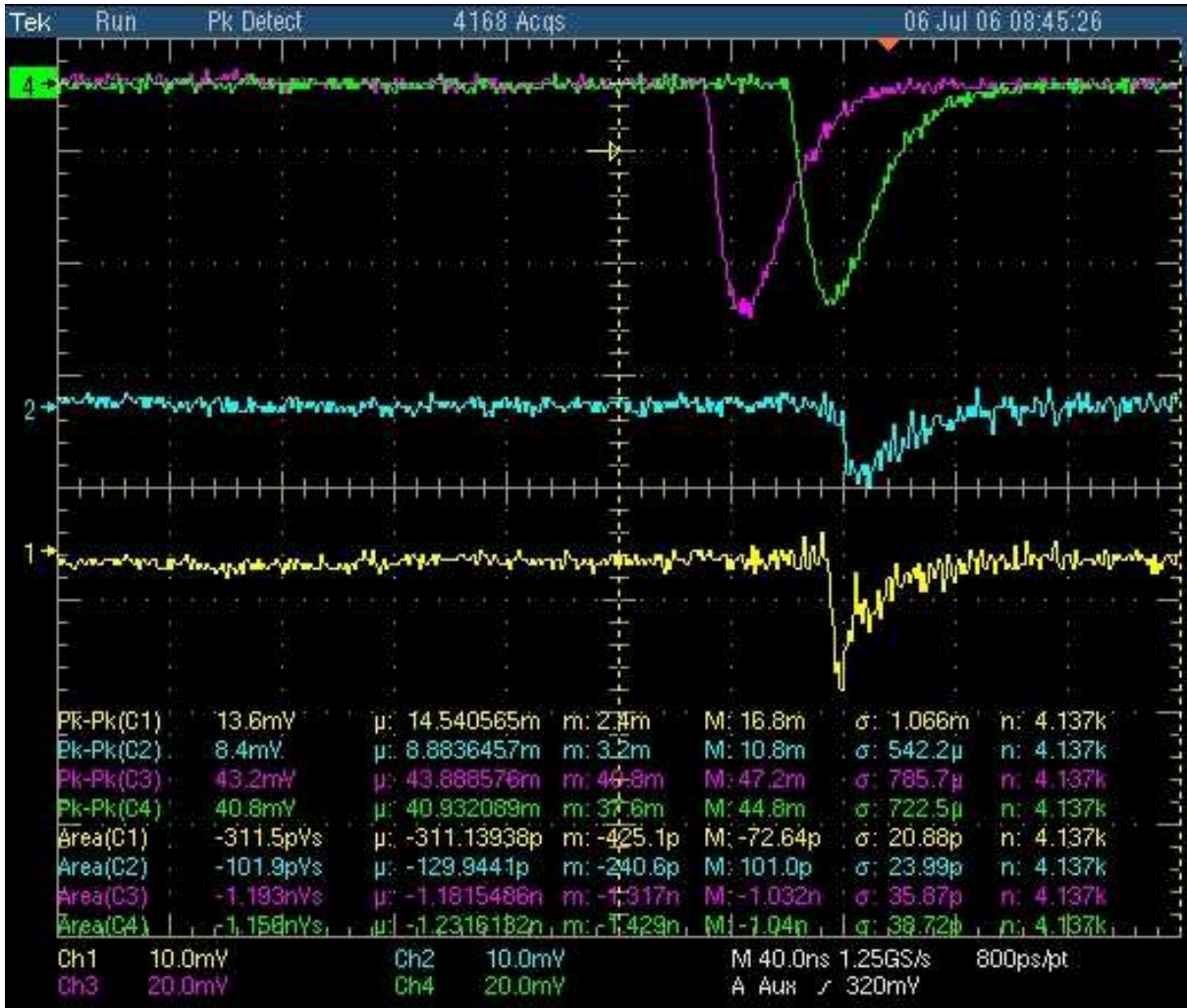
Figure 30: Signals from the WLS fiber displayed on the digital scope in configuration a ). The yellow and the blue signal are from the different ends of the fiber. Magenta and green belong to ICT1 and ICT2 (see Fig. 29). The wire of the Wirescanner was inserted at this measurement. The signal from ICT2 (green) is a little bit smaller than that from ICT1 (magenta). This indicates, that only few electrons of the bunch interacted with the wire and are not detected by ICT2. The signal from the upstream side of the fiber (Ch1) is slightly bigger than that from the downstream side (Ch2). Considering that the shower initiated by the wire passes the fiber before it's middle, the signal ratio is reasonable. For each channel the peak to peak (pk-pk) voltage and the area included by the signal is measured. These measurements are done between the cursors (indicated by dashed vertical lines: one in the middle, the other at the right border) and displayed on the screen. The mean ( \mu ) and the standard deviation ( \sigma ) are calculated based on the last 32 measurements and displayed. In addition the minimum (m) and maximum (M) value is shown.
