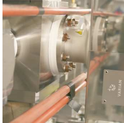
Figure 19: These plastic rods support the fibers whose flexible plastic tube is stuck to the opposite side of the rods.
