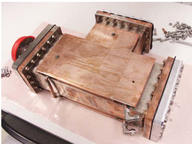
Figure 2: Photograph of the power combiner.
