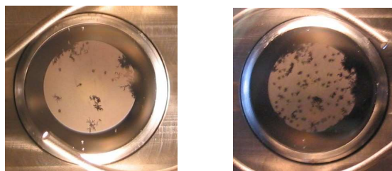
Figure 5: Damaged Cs 2 Te film on the cathode #60. Photographs were taken on March (left) and May (right) 2004.
