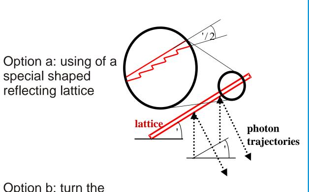
Option b: turn the streak camera that the photons hit the internal cathode simultaneously
