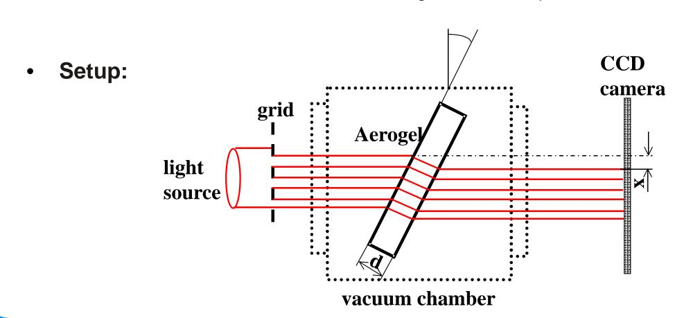
Result at different pressure: the refractive index of aerogel, with the same properties as that used in the ring imaging Cherenkov detector at the HERMES experiment in DESY Hamburg, is constant up till the pressure of 1 mbar, above it increases linearly
