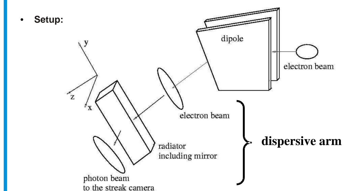
Radiator aerogel: mirror is tilted so that one part of the Cherenkov light is reflected perpendicular to the beam direction. Two electrons which crosses the radiator simultaneously produce photons with a time difference at the vacuum window, the time difference is represented with the angle
