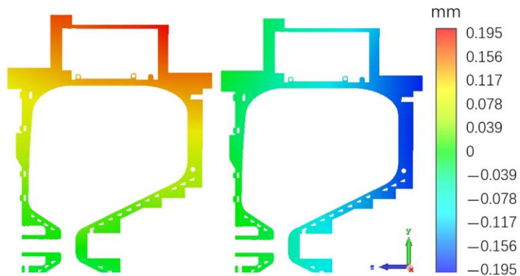
Radial (left) and axial (right) deformation of the VHF gun due to thermal expansion .
