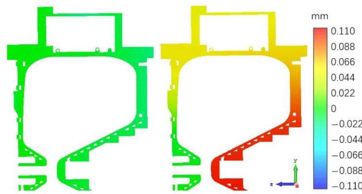
Radial (left) and axial (right) deformation of the VHF gun due to atmospheric pressure
