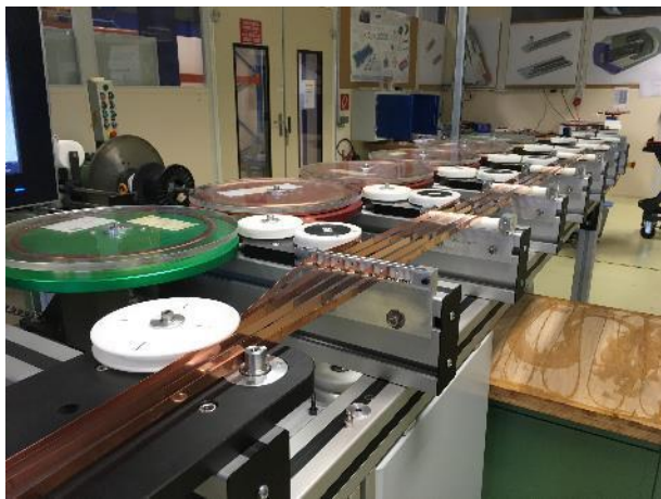
All 7 spools of the winding machine are operational and commissioned
