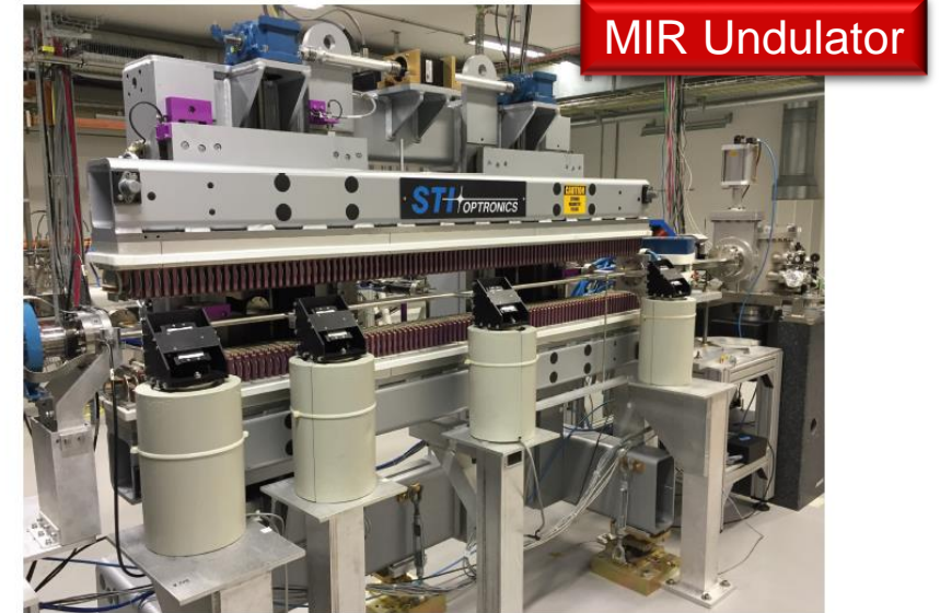
Figure 3. MIR FEL with undulator (center to left) and cavity end-mirror chambers (right) as of 2015.
