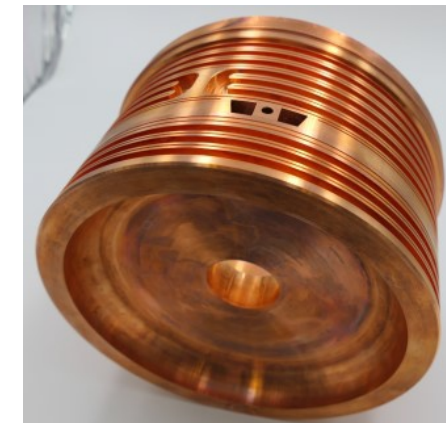
Central iris part with outer machining before brazing stainless steel jacket
