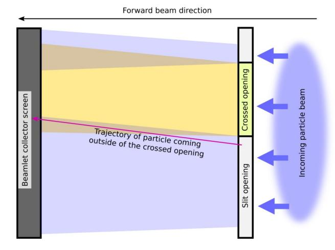
The beamlet crossing step has to isolate  $Q_0$  from  $Q_f$  as much as possible. The measured beamlet images of any vertical slit and any horizontal slit have separate foreign charges Q<sub>fx</sub> and Q<sub>fy</sub>. The pixel-wise minimum operation is used for beamlet crossing.
