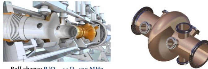
Bell shape: R/Q \sim 44 \Omega , 400 MHz
