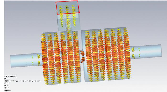
Field array plot in 4-cell S-band accelerating buncher
