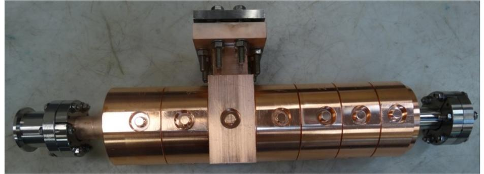
7-cell S-band accelerating buncher
