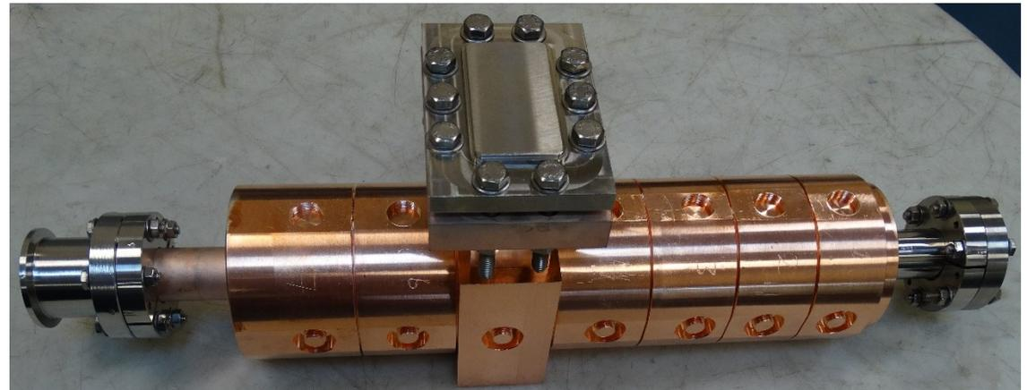
7-cell accelerating buncher during vacuum testing
