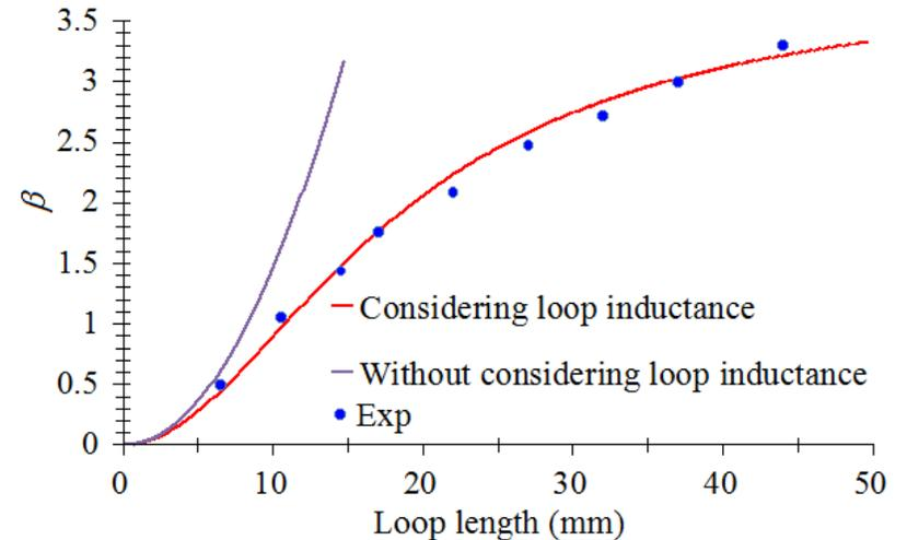
$\beta$  with length of loop for 476 MHz SHPB
