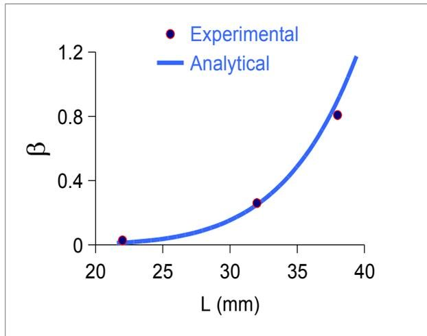
$\beta$  with slot length for 4-cell PWT linac
