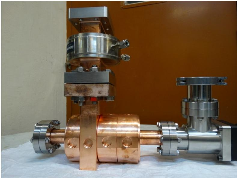
4-cell accelerating buncher during vacuum testing
