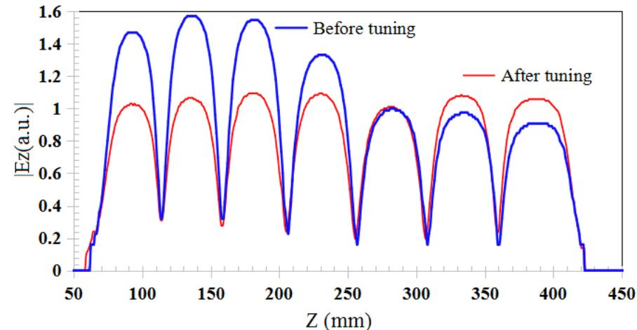
On-axis field profile in 7-cell S-band buncher before and after tuning ;
