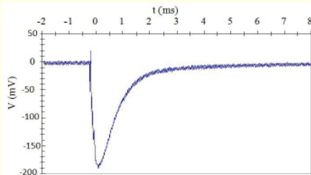
Typical bolometer signal with optical cavity length detuned
