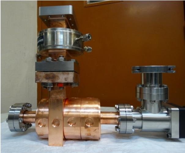
4-cell S-band accelerating buncher
