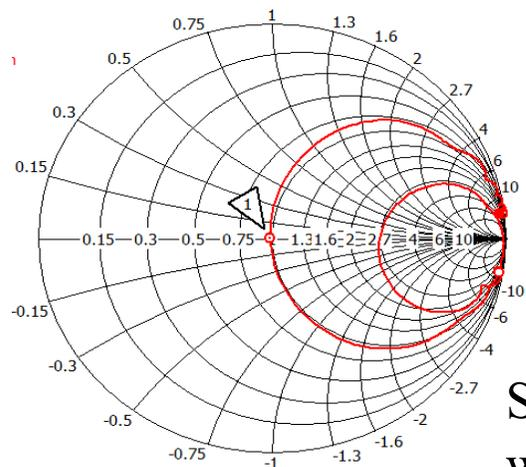
Smith Chart showing waveguide to cavity coupling
