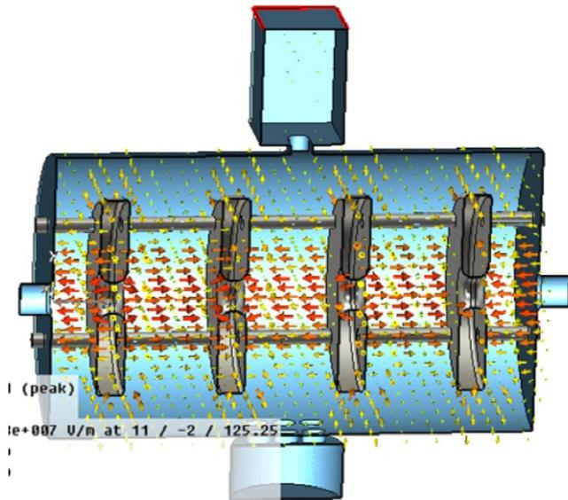
Field array plot in 4-cell PWT linac
