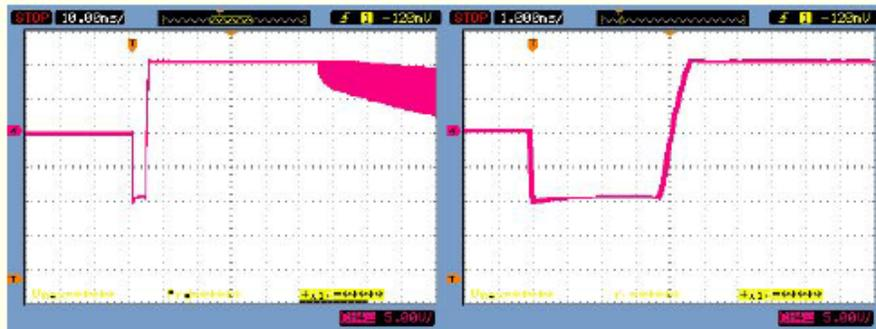
Typical bolometer signals showing a high degree of saturation with optical cavity tuned to design length
