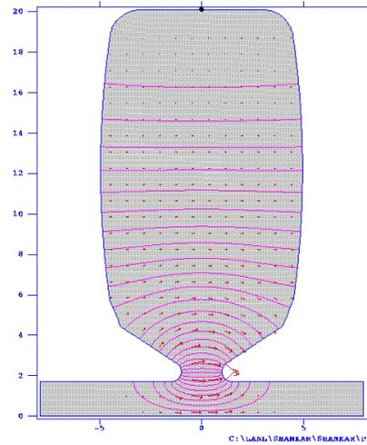
2D model of pre-buncher cavity
