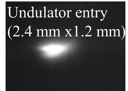
Electron beam signals at different locations
