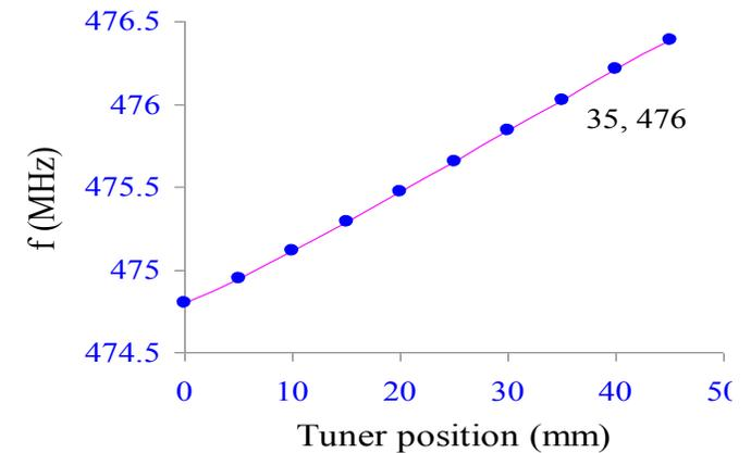
Resonant frequency v/s tuner positions
