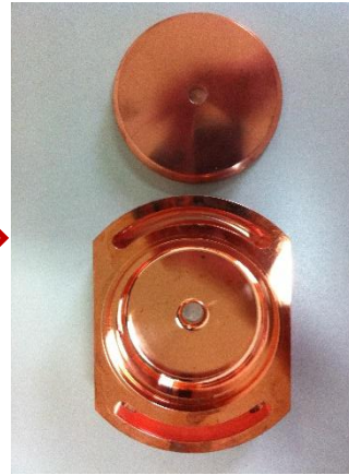
Copper cavity before welding
