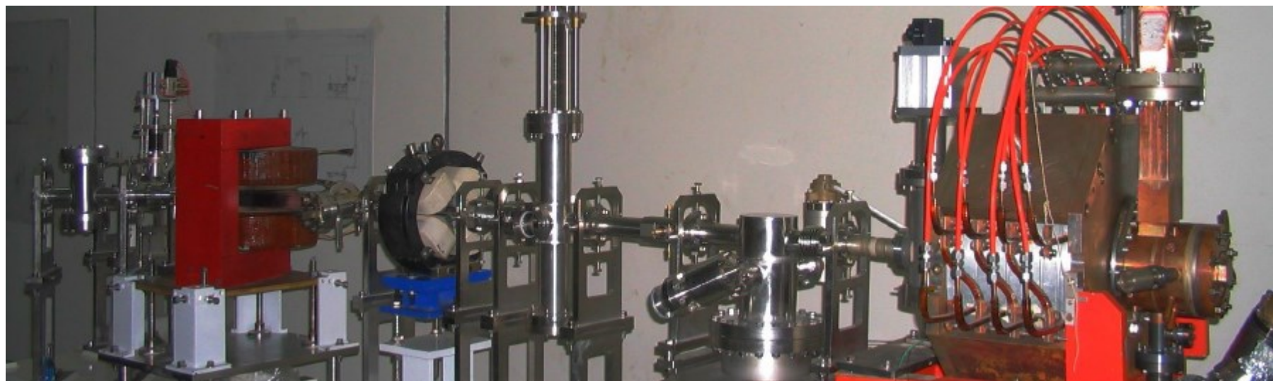
RF gun and the beam monitor system
