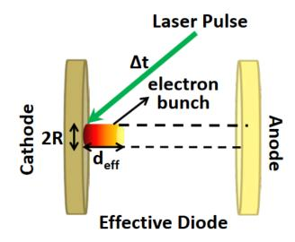
Steady state current limit described by Poisson equation  $\Delta \phi = -\frac{1}{\varepsilon_0} j_z \sqrt{\frac{m}{2e(\phi + E_0 z)}}$  $\frac{\partial \phi}{\partial z}|_{z=0,r \le R} = -E_0 \quad \phi(r,0) = 0$ Child-Langmuir Law<sup>[1]</sup> $J_{sat} = \frac{4\varepsilon_0}{9} \sqrt{\frac{2e}{m} \frac{V^{3/2}}{d^2}}$
