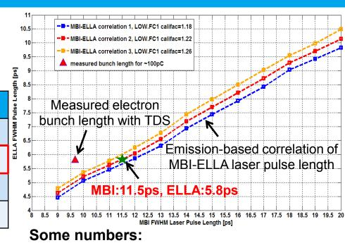
100pC measurements with TDS close to emission-based pulse length calculation, example:
