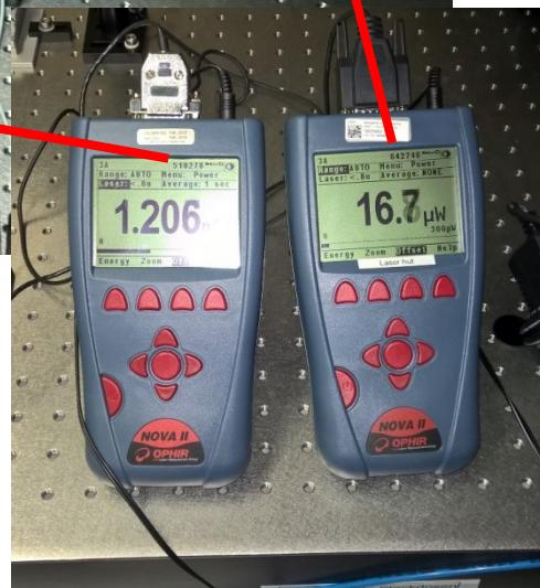
At Glen-Taylor-prism 50% of pulse energy (adjusted by  $\lambda/2$  wave plate) is reflected for reference measurement and 50 % is transmitted to laser window. Therefore simultaneous laser energy measurement of initial and transmitted laser pulses is possible!!!
