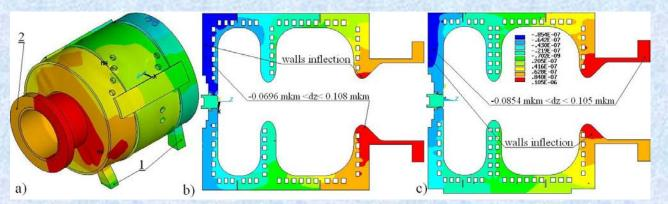
Deformations due to 2bar pressure in channels, df~-82 Hz.
