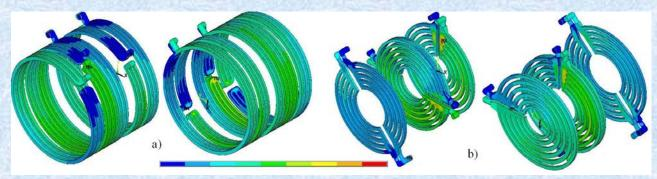
Temperature at the cooling channels (different projections). Channels works uniform – spread in output temperature is inside 2 C.
