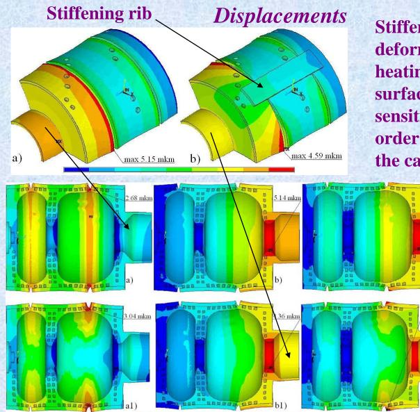
Stiffening ribs restrict cavity deformation due to pulsed heating, protect brazed surfaces, decrease frequency sensitivity and provide high order sextupole modulation in the cavity shape with ~µk scale.
