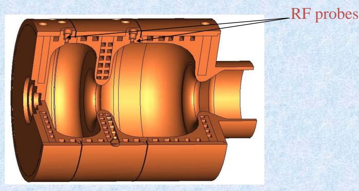
The key point in the improved cooling circuit is in internal flow distribution between small and more effective channels.
