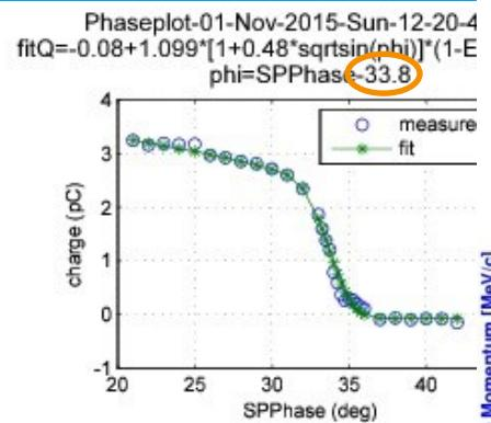
MS phase jitter=0.177deg; LaserEJitter=3.55%;
