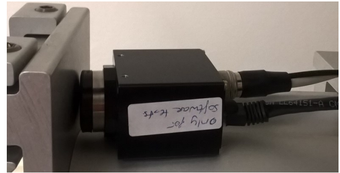
AVT (former Prosilica) camera connected to Ethernet and power/trigger cable
