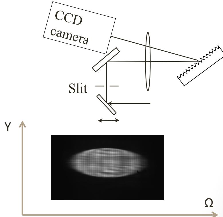
In this method we measure slice  $Y\Omega$  at different positions beam on the slit. It allows obtain 3D spectral intensity distribution
