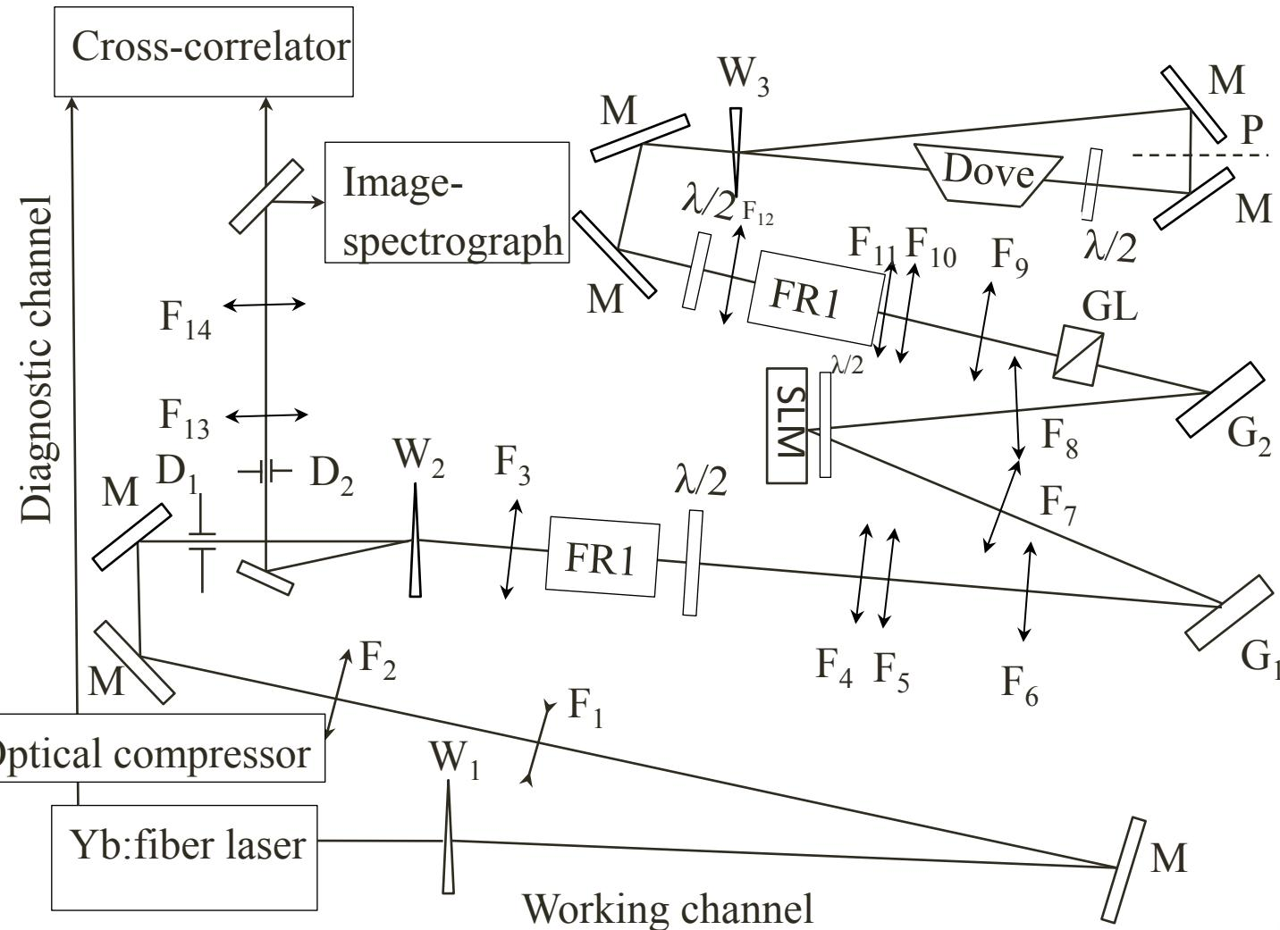
Output energy: 5.7nJ, pulse duration (FWHM): 41 ps, spectral bandwidth 7.3nm
