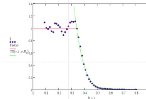
MatLab-generated input distribution for ASTRA with core + halo
