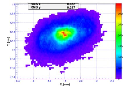
Measurement beam size at EMSY1
