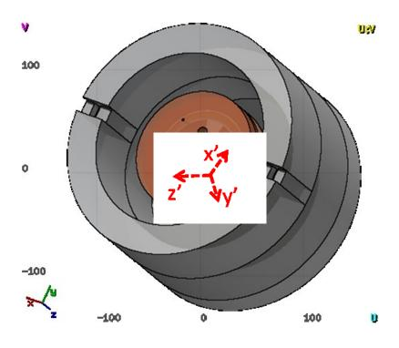
Each particle escaping the target volume needs to be "moved" to the position of the target within the cyclotron volume
