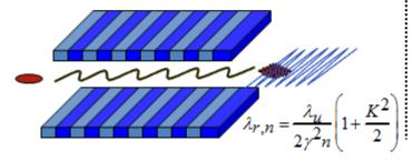
In an IFEL the electron beam absorbs energy from a radiation field.
