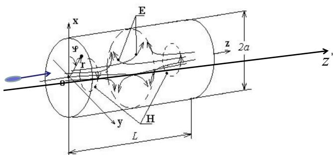
Booster steering procedure is to transport the beam by orbit where transverse deflections of particle are minimum depending on booster phase.
