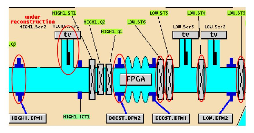
Degree of freedom is 4 (x, x', y, y') therefore for correct transportation of beam 4 steerers are needed.
