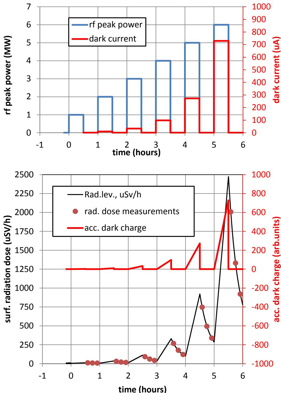
Main idea → several short (~30min) run periods with step increase of the peak rf power in the CDS, followed by short off periods (~30min), which should be used for surface dose rate measurements (e.g. 3 measurements 5;15;25 min)
