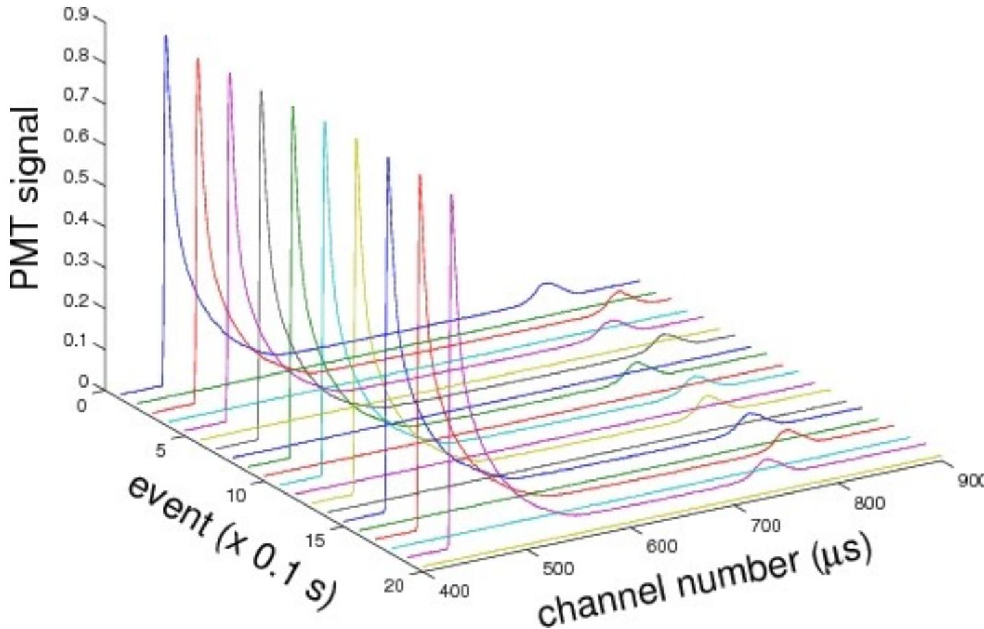
1. Regular PMT signal is missing for each second event (not 0, but noise!) .
