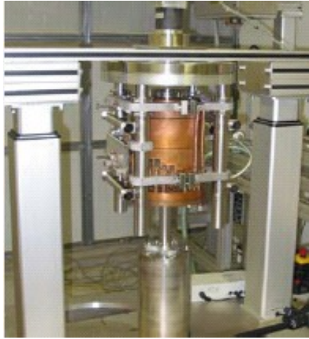
Vertical cleaning setup with 110° rotating nozzle.
