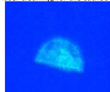
The QE image for a laser spot half on a cleaned area and half on an uncleaned area. The image was taken at a screen located about 1.43 m downstream of the gun, with a 20 pC bunch charge.
