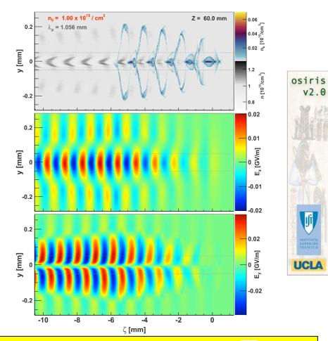
Expected energy modulation  $\approx 600 \text{ keV}$ . PITZ beam energy spread as low as  $\approx 60 \text{ keV}$ . Resolution of TDS/HEDA2: 10keV and 100µm (Malyutin et al. "Simulation of the Longitudinal Phase Space Measurements With the Transverse Deflecting Structure at PITZ", *Proc. of IPAC 2012, MOPPP034*  $\rightarrow$  Measurable
