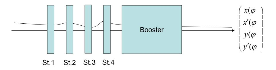
$$\begin{vmatrix} I_1 \\ I_2 \\ I_3 \end{vmatrix} \rightarrow \text{? to provide after booster} \begin{vmatrix} x_{\text{max}} - x_{\text{min}} | < x_{\text{tol}} \\ x'_{\text{max}} - x'_{\text{min}} | < x'_{\text{tol}} \\ y_{\text{max}} - y_{\text{min}} | < y_{\text{tol}} \\ y'_{\text{max}} - y'_{\text{min}} | < y'_{\text{tol}} \end{vmatrix}$$
