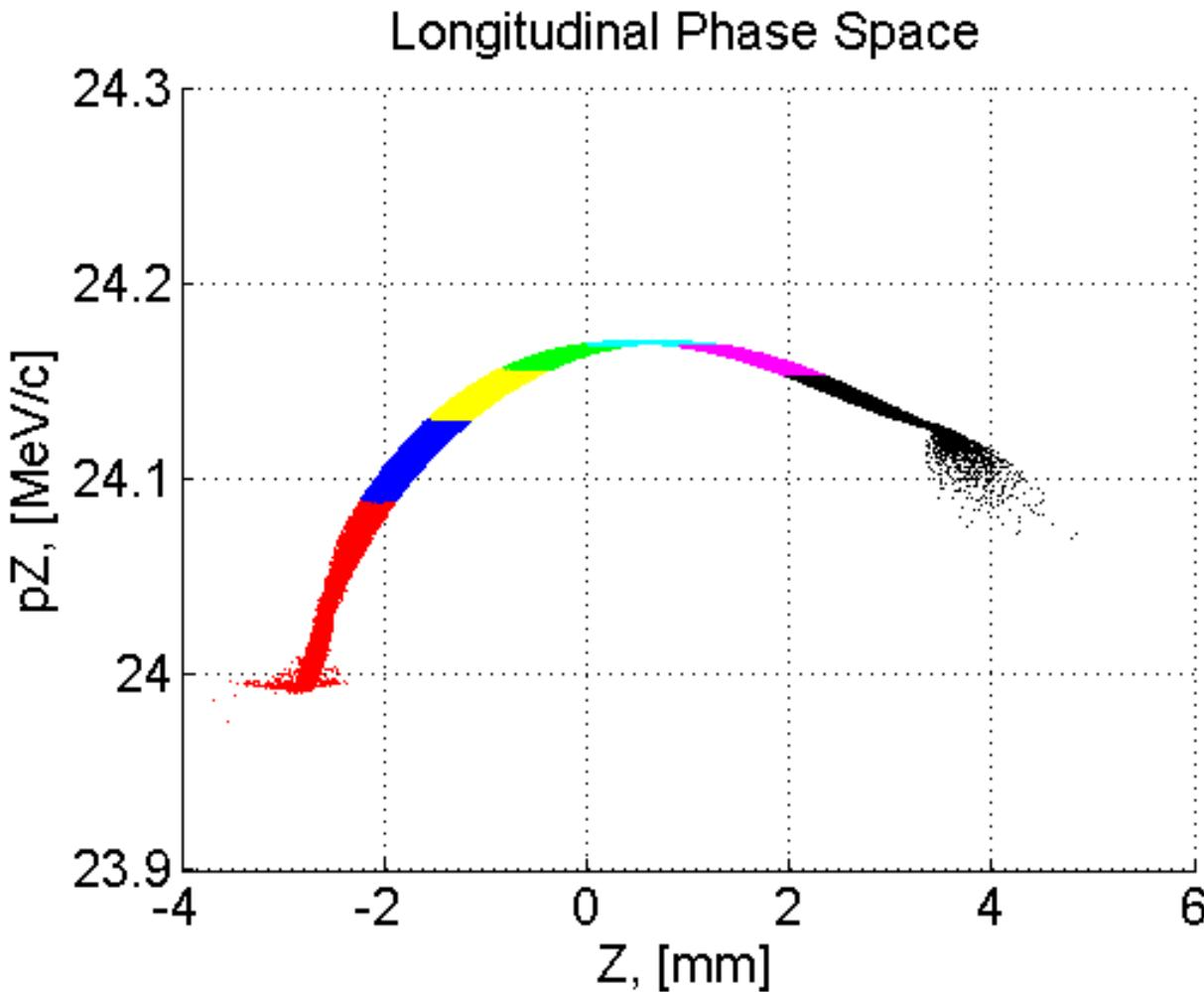
Example of longitudinal phase space for 100pC bunch charge.
