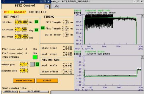
700 us pulse duration. High radiation around HEDA1. A lot of electron detector in WG2 ILs correlated with PD in WG1. Looks like we have a problem with WG2 RF window, may be we have to open the system for inspection
